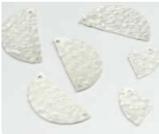
6. Pickle until the oxidation is gone, then repeat until no further oxidation is possible, then pickle one last time, rinse and air dry
